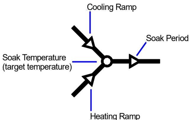
An KCR32C firing segment comprises a ramp followed by a soak period. Two segments can be used for simple firing (biscuit firing for example) or several segments can be used per program for complex firing (crystal glazing or glass-making for example).
